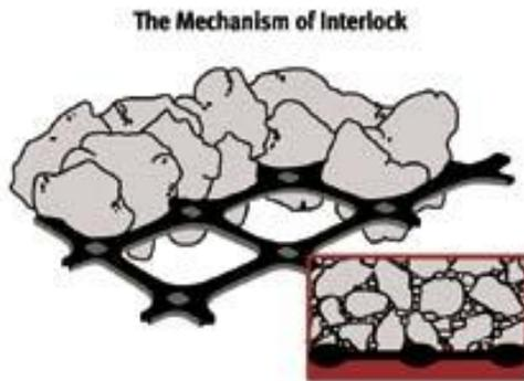
Fig 2: Mechanism of Geogrid Reinforcement
