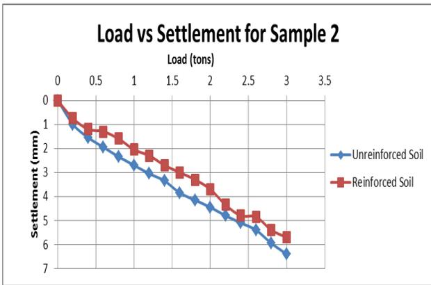
Fig 11: Load vs Settlement Curve for Sample 2
