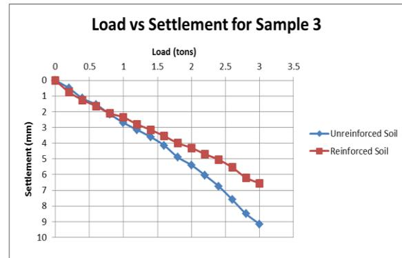
Fig 12: Load vs Settlement Curve for Sample 3
