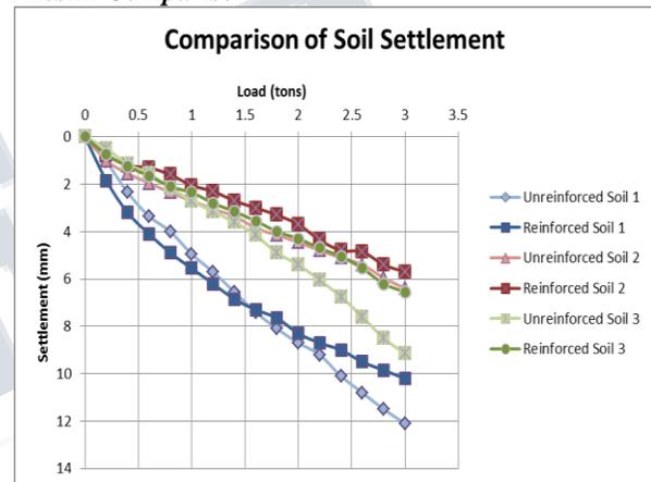
Fig 13: Load Settlement Comparison Curve for all 3 Samples
