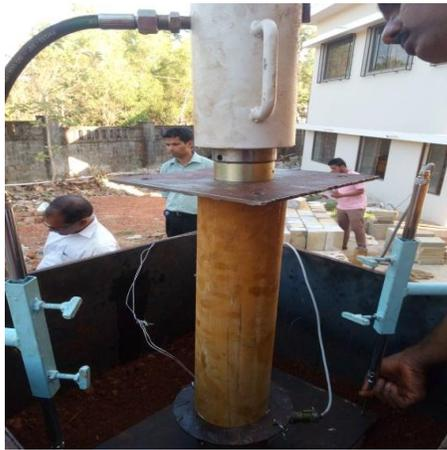
Fig 9: Loading arrangement of Soil
