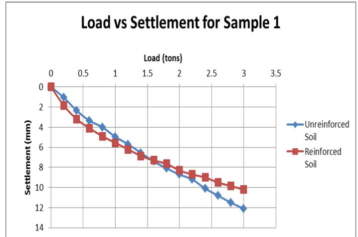
Fig 10: Load vs Settlement Curve for Sample 1
