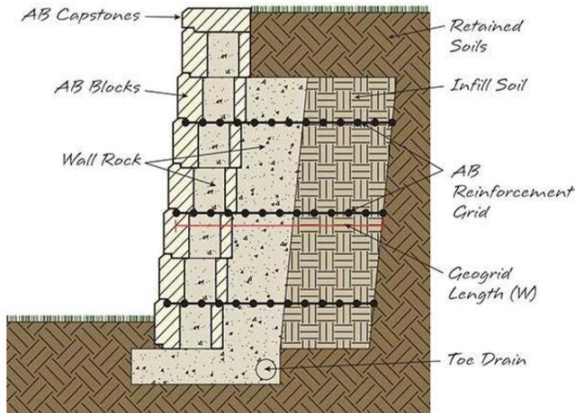
**Fig 4 Geogrid for Retaining Wall**
