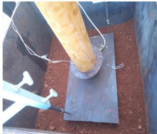
**Fig 8: Setting of LVDT**
