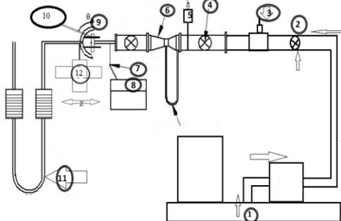
**Fig.1. Experimental setup (1) ELGI Airmate, Air screw compressor with refrigeration unit with capacity of  $1.1\text{m}^3/\text{min}$  and maximum supply pressure of 7 bars), (2) ball valve (3) pressure regulator, (4) flow control valves, (5) pressure gauge, (6) venturimeter, (7) calibrated K-type thermocouple, (8) millivtmeter, (9) curved surface, (10) confinement plates, (11) calibrated double bulb micro mano meter (12) calibrated compound sliding table**
