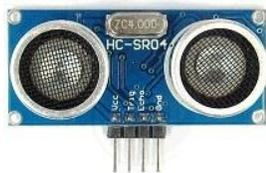
Fig 3.3 : Ultrasonic sensor
