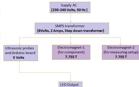
Fig 5 Block Diagram of Automation System
