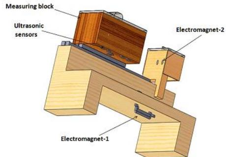
Fig 4: Final Assembly of Inspection Setup
