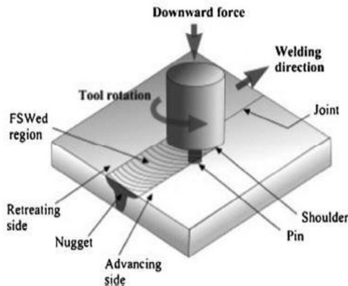
Fig 1: Friction Stir Welding Process
