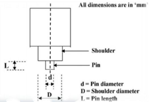
Fig. 2: FSW tool dimensions
