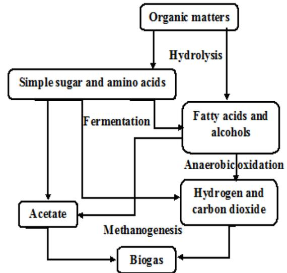
Figure 5: Process flow diagram for anaerobic digestion
