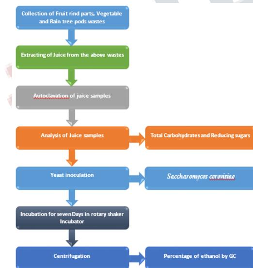
Figure 7: Process flow diagram for Bioethanol production
