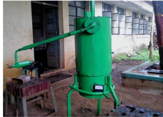
Figure 8: Pyrolysis unit
