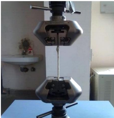
Figure-1 Tensile test specimen setup
