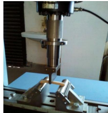
Figure 3- Flexural test set up with 80mm span length
