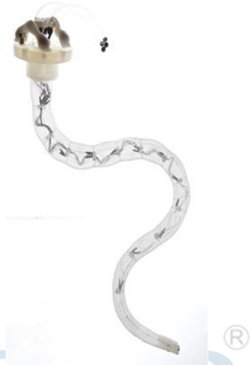
Figure 2. Flexible octopus-like robot arm, composed by a braided sheath actuated by SMA springs (photo by Massimo Brega, The Lighthouse).
