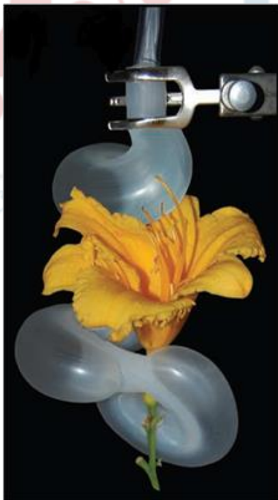
Figure 1. Pneumatic tentacle-like soft manipulator (Martinez et al., 2013) (reproduced with permission from John Wiley and Sons).
