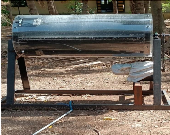
Figure 5.1. Actual setup of conductive rotating drum type solar dryer
